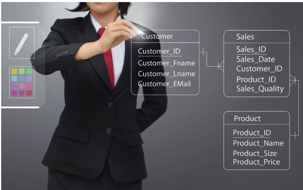
■ Example of an entity–relationship diagram (ERD) for a relational database
